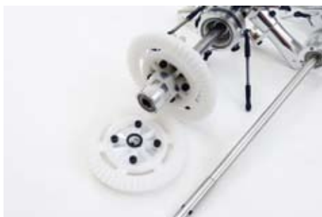
Bearing block with 10 mm bearing on the lower shaft and 8 mm bearing waiting for the main shaft
