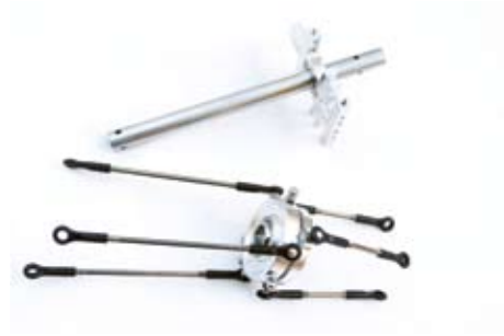
Lower swashplate has the same size upper and lower sections so both swashplates tilt the same amount
