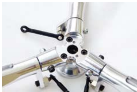
Underside of the lower hub showing the screws holding it to the cone shaped bearing holder
