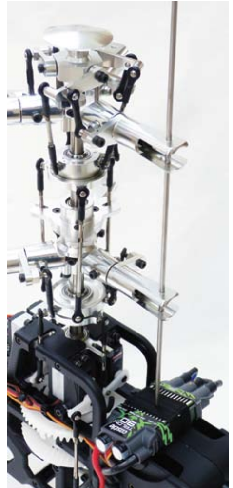
The bevel gear sits slightly outside the main gears, the mesh is correct and if any wear occurs, the pinion could be shimmed to tighten the mesh
