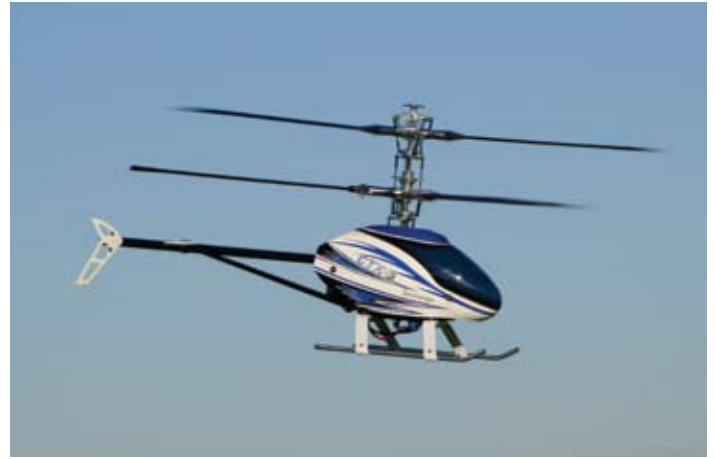
Pushing into forward flight shows the pendulum effect – you can see the upper rotor head leading
