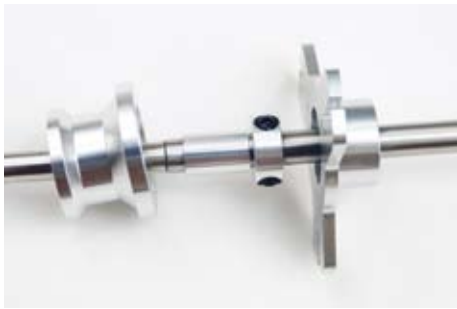
Main shaft with a collar secured using tapped holes in the shaft; note the reduction in diameter giving clearance for the lower shaft that runs over it
