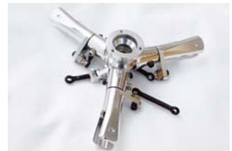
You can just see the 8 mm bearing that carries the main shaft
