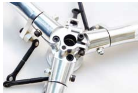
The swashplate driver covers a fixing screw
