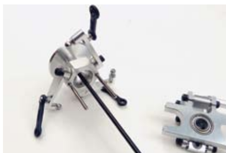
The mixer arms on the yaw spider are ball raced and the guide pins slide into the rotor hub
