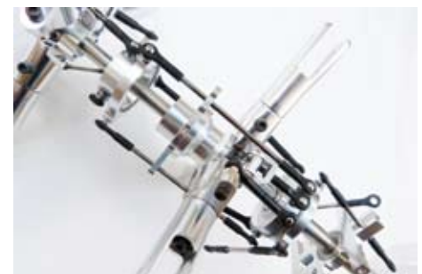
Lower rotor head showing the bearing blocks that carry the 8 mm mainshaft and 10 mm lower shaft
