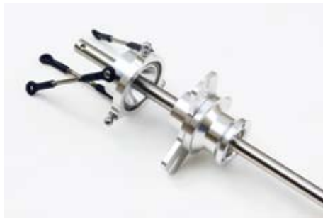
The secured collar is between those two bearing holders that are thus fixed in position
