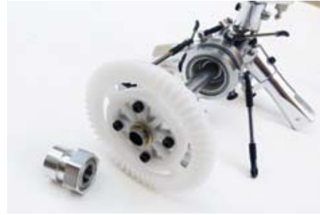
Lower shaft assembly with its 53 tooth main gear
