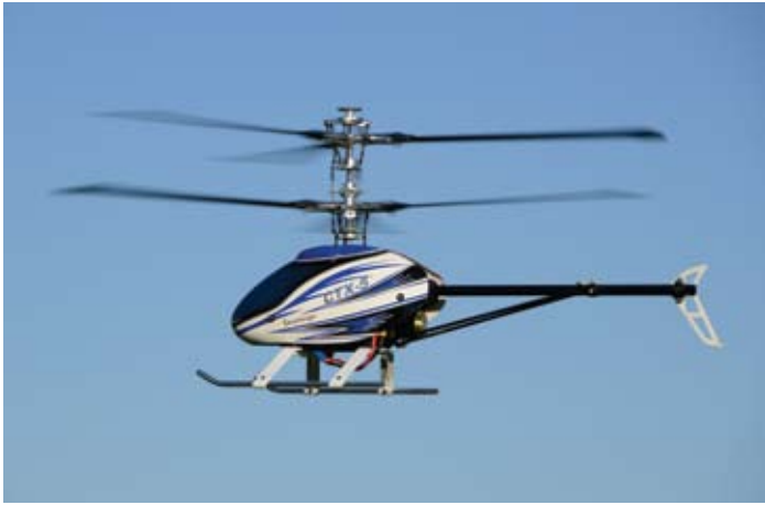
Seeing two rotor heads and swashplates above the canopy takes a little getting used to
