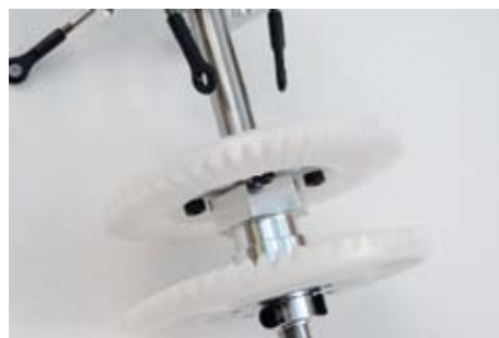
The hex shaped bearing block locates into the side frames so it can't rotate
