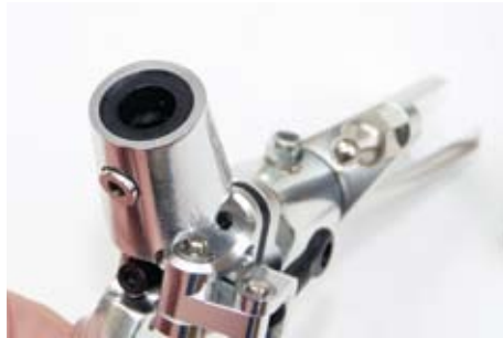
There are two of these hard dampers, one either side of the securing screw that acts as a flapping fulcrum point
