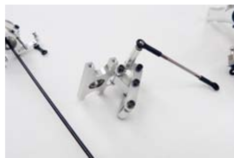
Lower bearing block supports the main shaft, as well as the yaw pitch assembly
