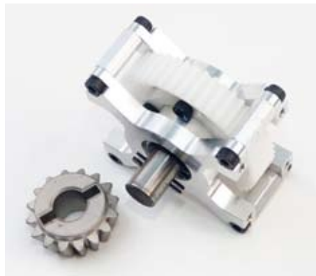
The bevel gear sits slightly outside the main gears, the mesh is correct and if any wear occurs, the pinion could be shimmed to tighten the mesh
