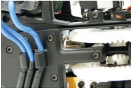
Reduction gearing – the bevel gear doesn't need a fixing screw
