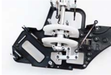
The plastic used is quite soft but the hex spacers and bearing blocks produce a solid assembly – note the hexagonal section prevents it rotating
