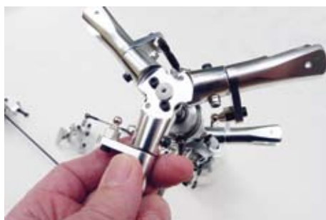
Upper rotor head with the plastic guide and the holes for the spider guide pins
